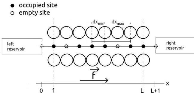
FIG. 2. Schematic diagram showing the pore modeled as a one-dimensional lattice. The external portions of the polymer are modeled as particle reservoirs at equilibrium. The particles hop preferentially to the right under the influence of the external force field  $\vec{f}$ .
